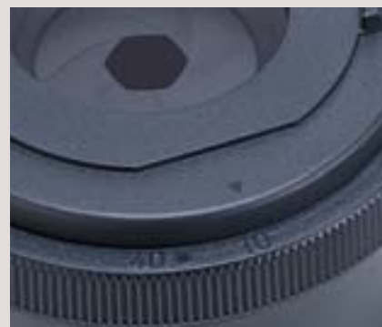
Field diaphragm with position-guide markings
